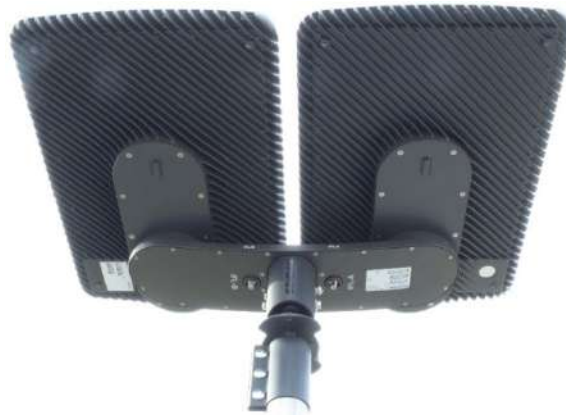
Figure 16: ODU mounted to mast adapter
