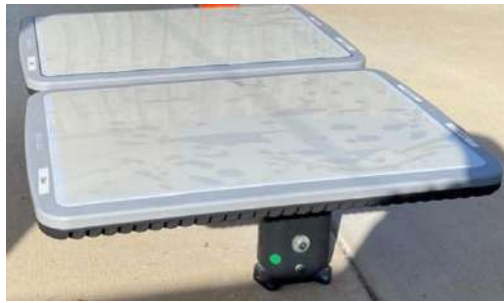
Figure 13: ODU installed with penetrating mount
