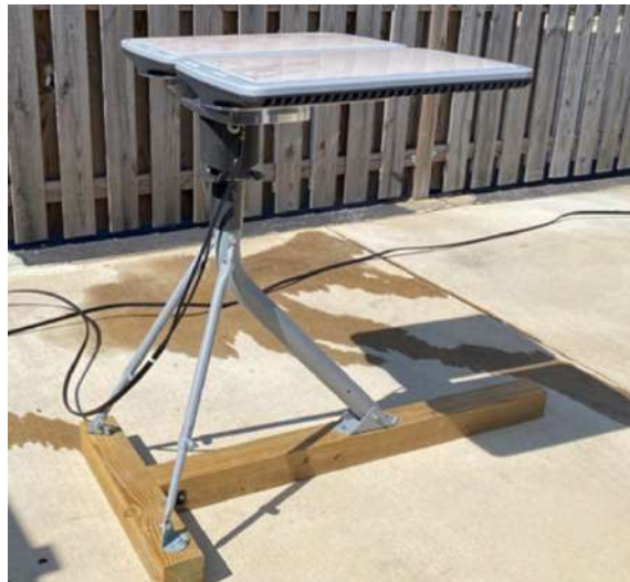
Figure 20: ODU mounted to trimast with mast adapter
