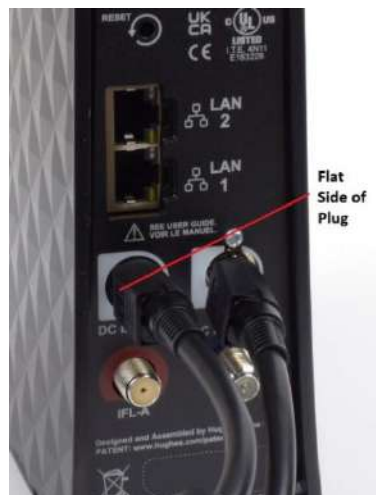
Figure 26: Proper power cord orientation
